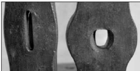
The result of the second upsetting. Note the shape of the hole in the back differs from the front.
