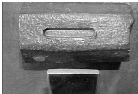
Checking the location of the punch with the business end of the punch shown.
