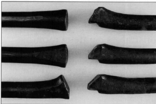
Steps in forming the scarf for forging.
