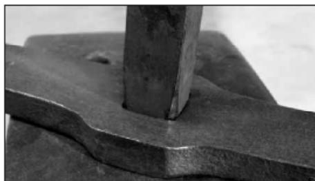
Return to drifting the hole. Remember to work from both sides of the material.
