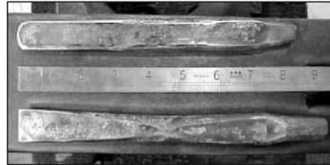
Check the stock after the first blow with the punch to see if it is correctly aligned with the barstock.
