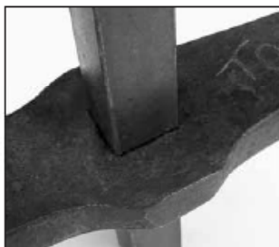
The square blocking complete with a taper to the end of the bar and a tenon drawn.
