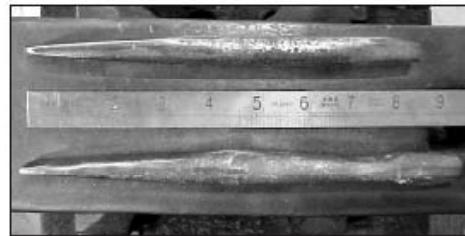
Drift (upper) and punch shown from the front and side.
