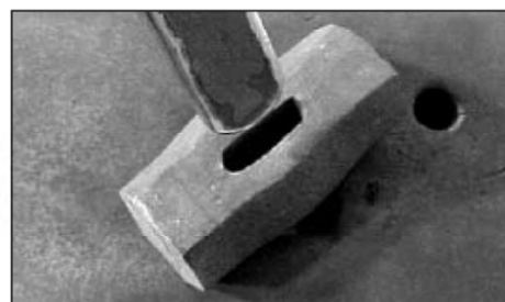
Starting to drift over the hardie hole.
