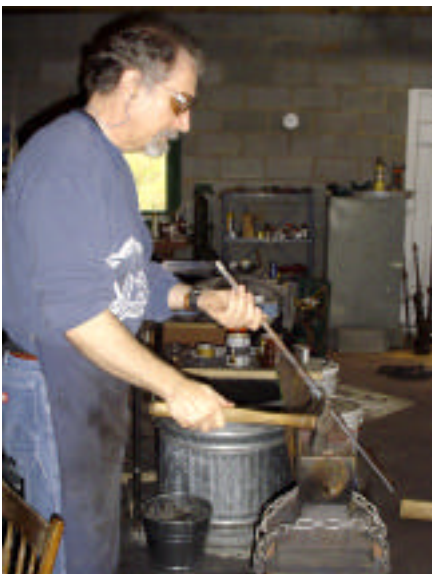
15. Sighting down the bar to locate bends and help keep it straight.
