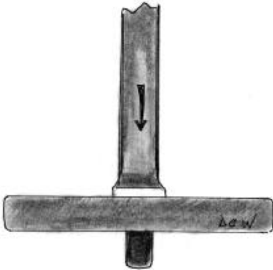
#7. Using the bolster plate
