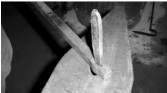
Supporting the bar with the edges of the pritchel hole
