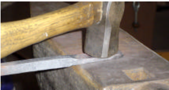
5-7. Working the face of the bar in the middle of the anvil, working the edge of the bar, and working the face with the unforged bar off the anvil.
