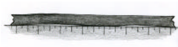
12. Deviation from straight on left because of bend, on right because of narrow portion in the bar.
