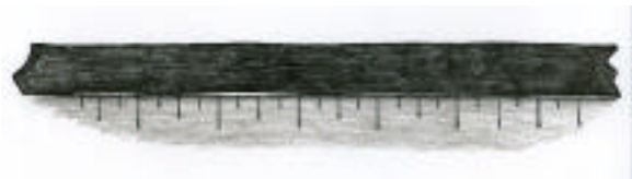
11. Checking with a straightedge—dramatic deviation on left, close approximation on right.
