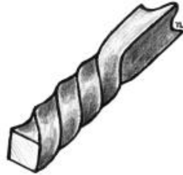
11. Forging dynamics of twisting.
