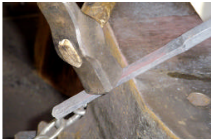
Photo 14: Scraping along a sharp anvil corner to get rid of scale before forging. Use the hammer head to apply downward pressure.
