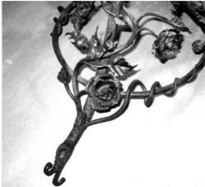
A forge welded sample from Cyril Colnik
