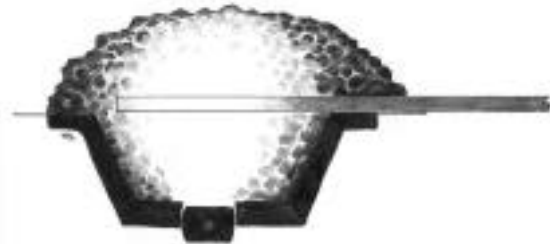
3. Bar placed in the fire horizontally, with the tip beyond the hottest part of the fire
