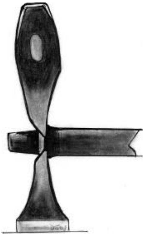
#5. Marking the second side of the bar
