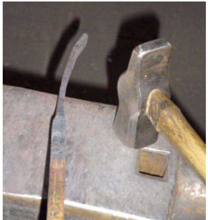
16. Major problems like this are easy to see sighting down the bar, but more subtle ones become evident too. Can you see the 2 sharper bends in this bar?
