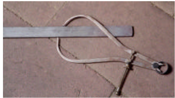
8-9. Top— proper use of the caliper with points opposite each other. Bottom photo shows a false reading.
