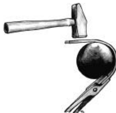
8. Manipulation of stock for bending on the horn.
