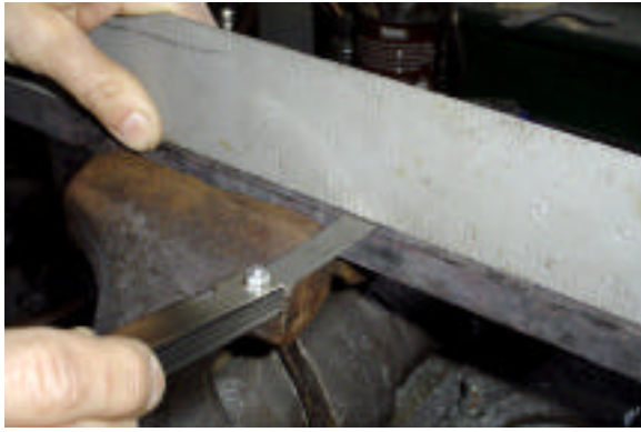
14. Testing with the feeler gauge.
