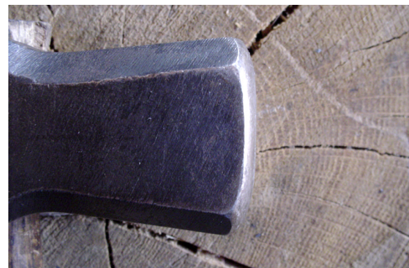
2. Properly ground hammer face
